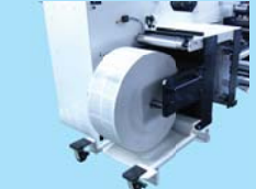
Unwind Front Gate is locked in position to provide stability and support to the unwind shaft
