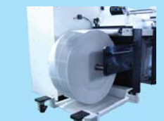
The unwind shaft is raised into the running position, just clear of the floor or cart.
