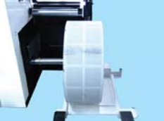
Unwind shaft lowered to level of core in new roll and new roll being loaded
